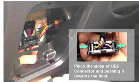
Figure 2: Removing OBD Connector and Installation
